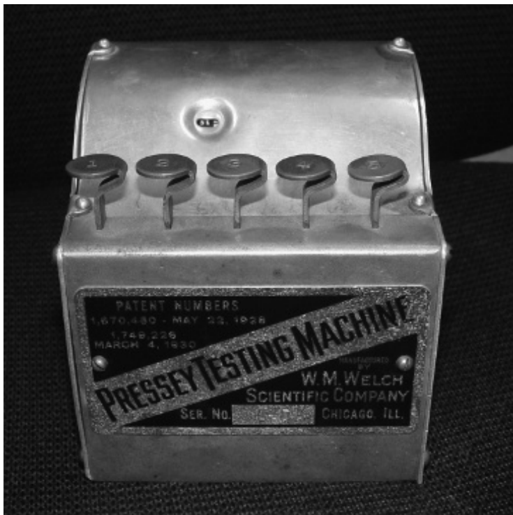
Figure 3.5 Pressey's Testing Machine.
